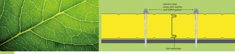
The Metfiber® Eco Wall panel with glass wool core fulfils all the requirements for non-combustible building materials. The glass wool used in this product consists of 80% recycled material, contributing significantly to the saving of natural resources and making the product an ecological building material. The deadweight of the panel is distinctly lower than that of conventional sandwich panels with rock wool insulation core, hence enabling an easier,
